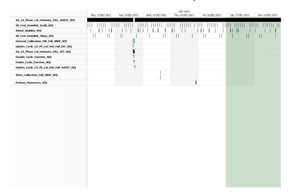
This week contained a **NIR** External Calibration on the 13/12/11 with **ETO** at **16:26:00 UTC** + **PMS Offset Calibration** on the 14/12/11, and an Orbit Control Manoeuvre (OCM) programmed on the 15/12/11 at 21:55:51 UTC. Besides, X\_Band passes over ESAC and Svalbard.
