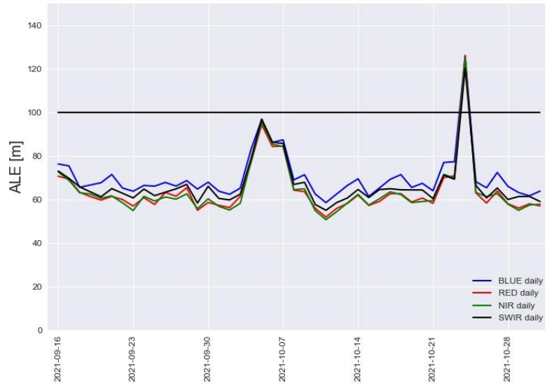
Figure 21: Daily average location error in the period from 16/09/2021 – 31/10/2021 (left) and the average daily compliance of all spectral bands (right).
