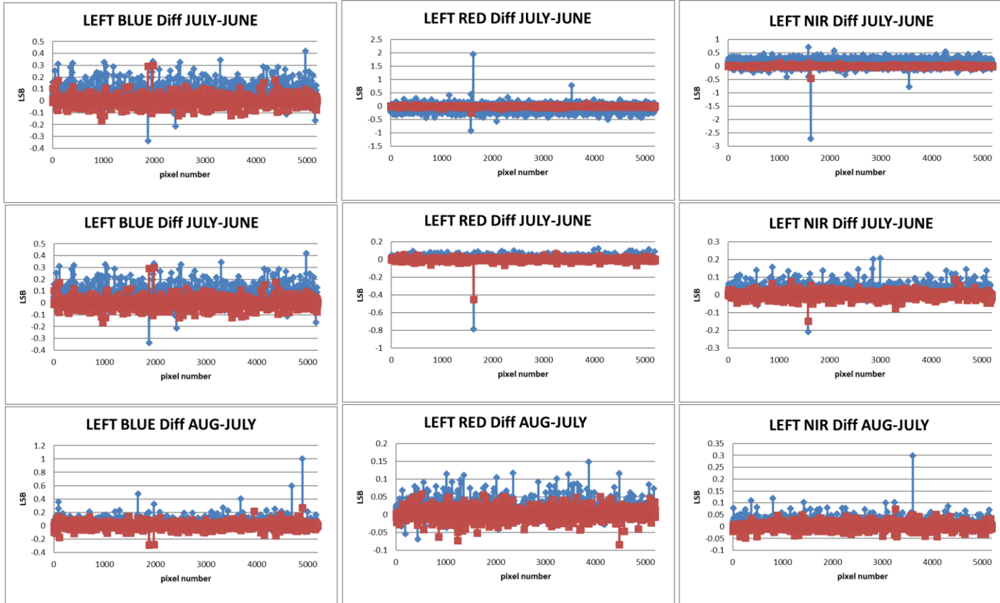
Figure 12. LEFT camera VNIR: Monthly difference (MAY-AUG2019) in dark current (Blue) and standard deviation (Red) of the monthly averaged
