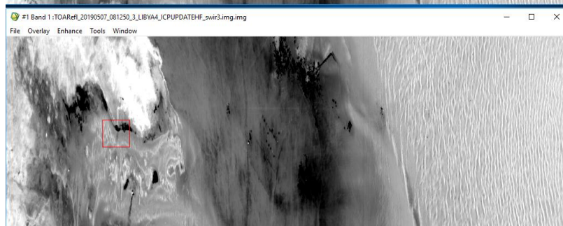
Figure 23. Visual assessments of the improvement of the scene uniformity through application of the yaw retrieved updates to the equalisation coefficients. (Note :black vertical lines are known BAD pixels). Results for RIGHT SWIR3.
