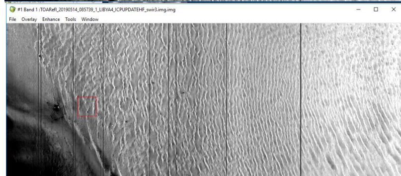
Figure 20. Visual assessments of the improvement of the scene uniformity through application of the yaw retrieved updates to the equalisation coefficients. (Note :black vertical lines are known BAD pixels). Results for LEFT SWIR3.
