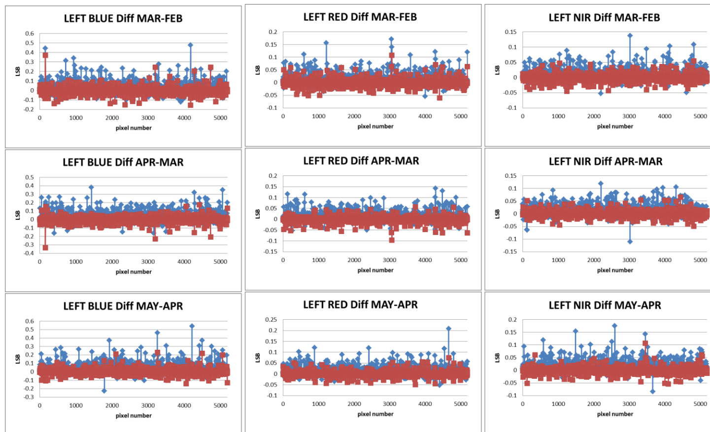
Figure 13. LEFT camera VNIR: Monthly difference (Feb to May 2017) in dark current (Blue) and standard deviation (Red) of the monthly averaged results.
