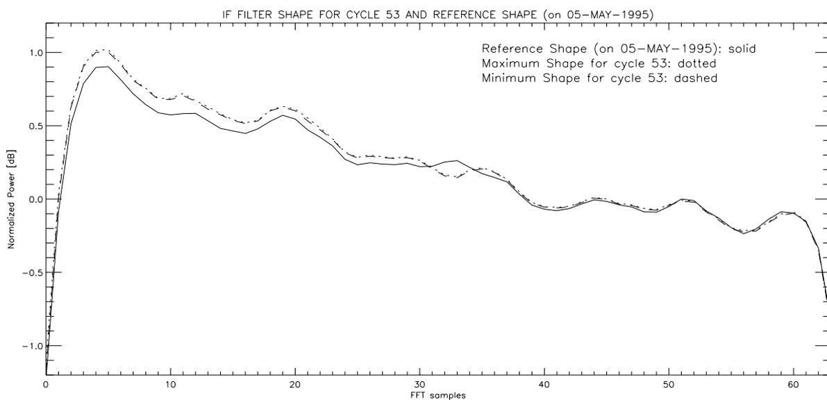
The two pages reported afterwards document trends of the IF filter characteristics difference respect to the reference, for each of the 64 FFT samples averages over cycles have been calculated.
