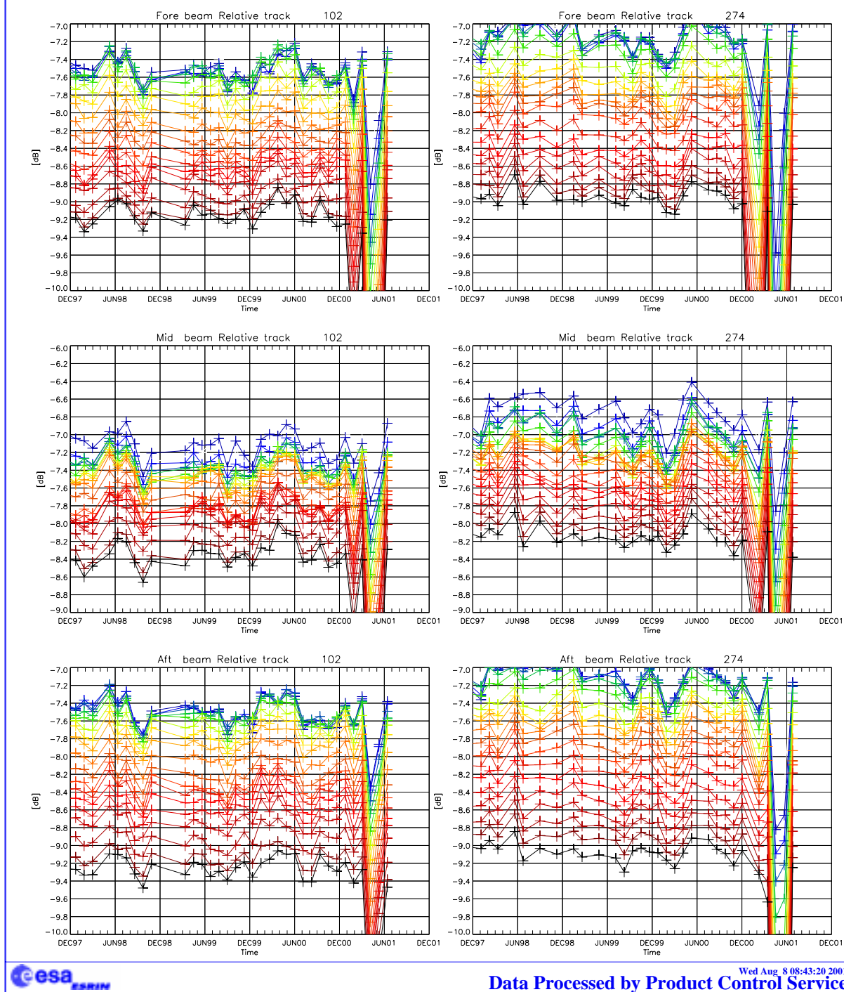
FIGURE 16. Sigma nought over the test area: ascending passes relative tracks 102 (left panels) and 274 (right panels); all nodes across the swath (since December 1997).
