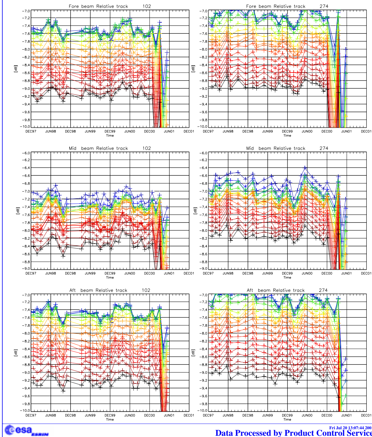
FIGURE 23. Sigma nought over the test area: ascending passes relative tracks 102 (left panels) and 274 (right panels); all nodes across the swath (since December 1997).
