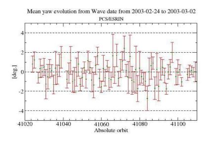
**Figure 1** Mean Yaw Evolution from Wave (green) and Scatterometer Data (blue)
