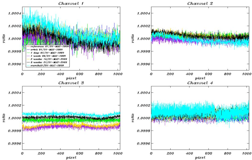
Fig. 5-8: Dark current ratios (constant part) channel 1-4 during May 2009. Reference Spectrum used: Orbit 37478, 01-May-2009.
