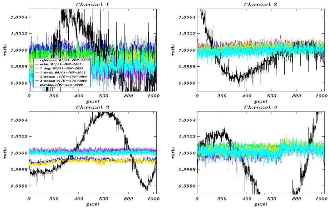
Fig. 5-10: Dark current ratios (constant part) channel 1-4 during June 2009. Reference Spectrum used: Orbit 37921, 01-June-2009
