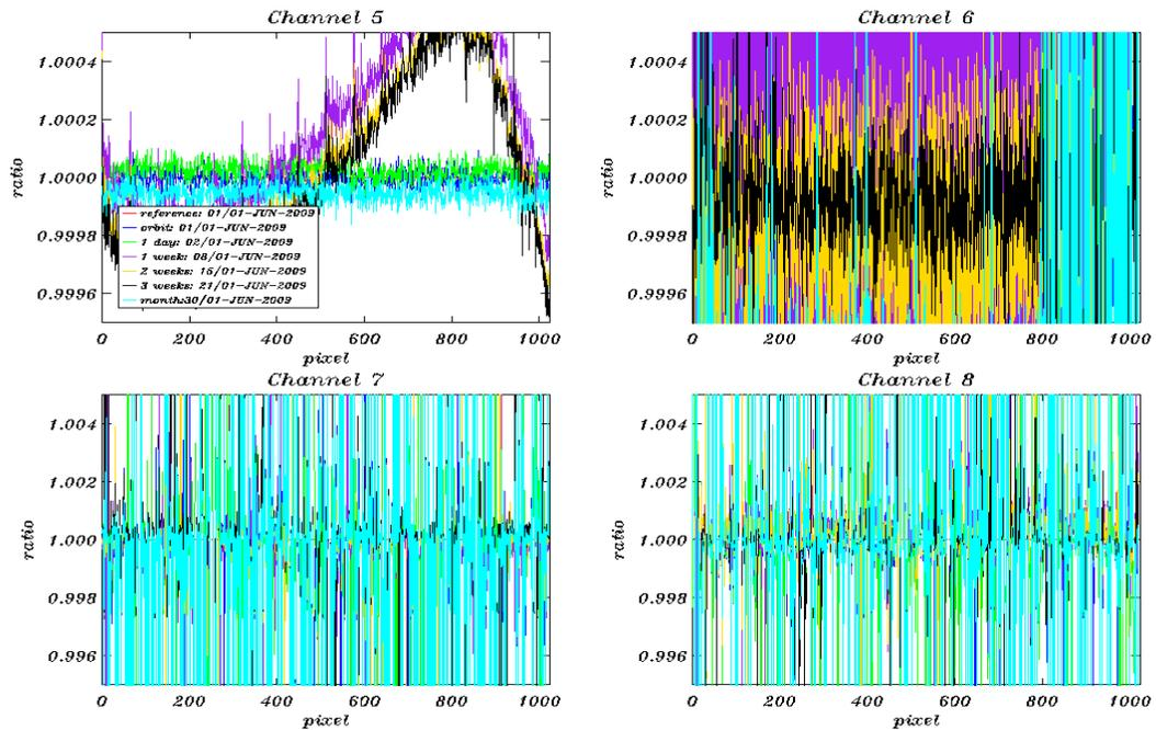
Fig. 5-11: Dark current ratios (constant part) channel 5-8 during June 2009. Reference Spectrum used: Orbit 37921, 01-June-2009.
