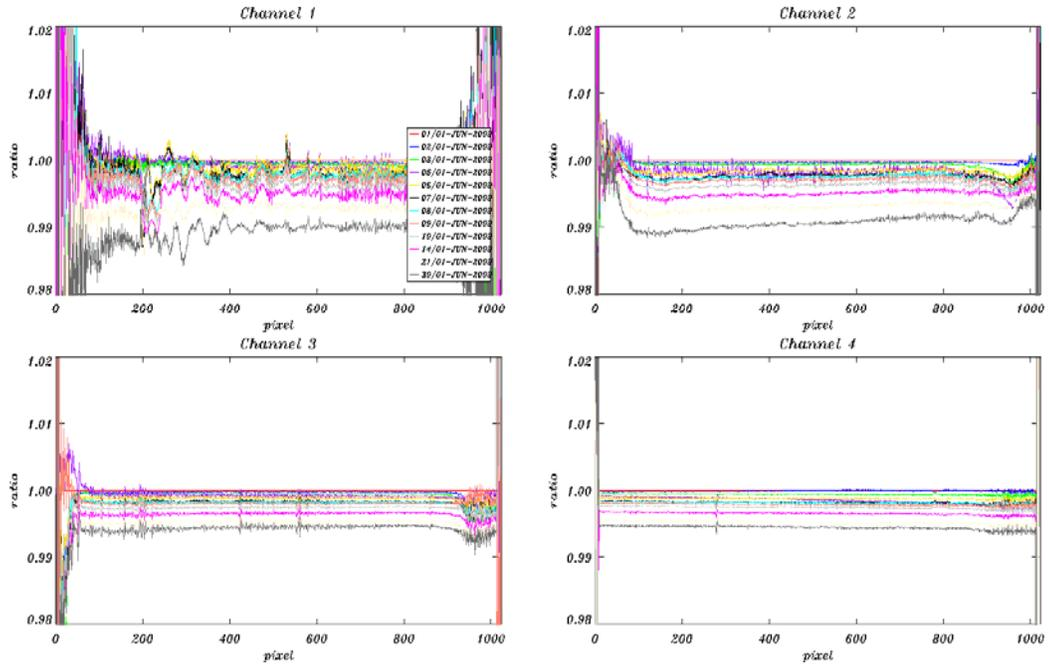
Fig. 5-4: SMR ratios per detector channel 1-4 (changes during June 2009).
