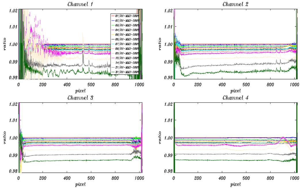
Fig. 5-2: SMR ratios per detector channel 1-4 (changes during May 2009).
