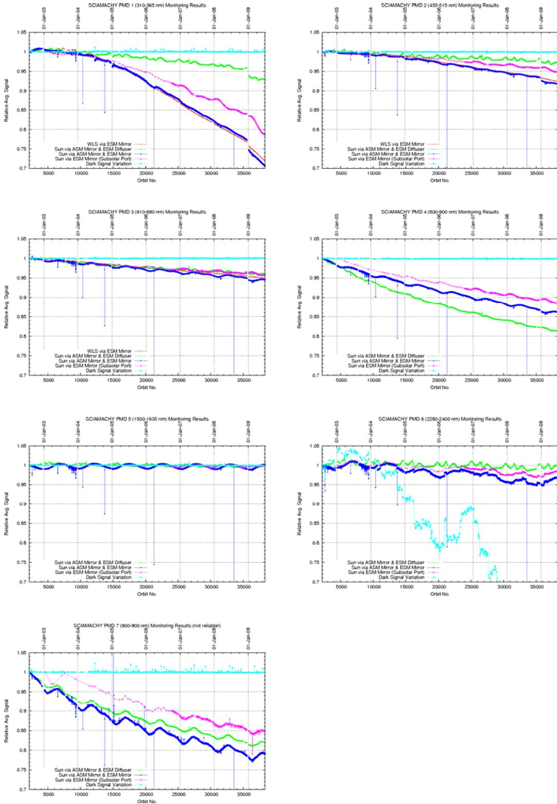
Fig. 3.12: PMD monitoring results August 2002 to June 2009.
