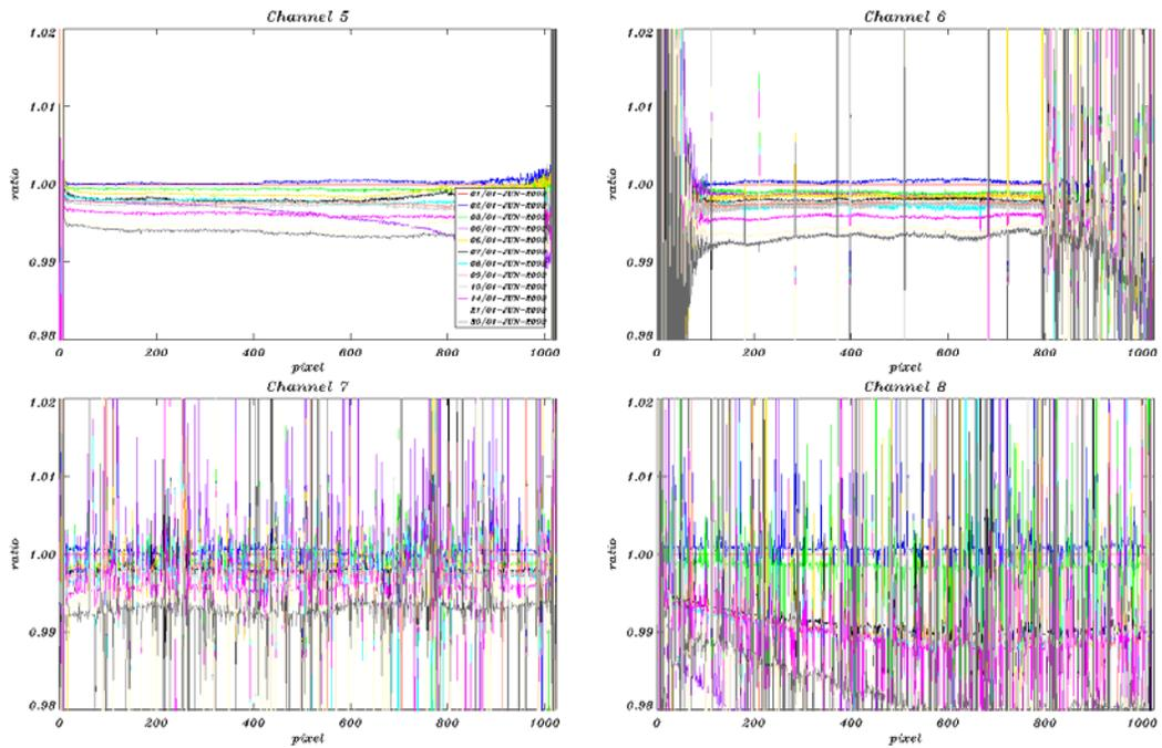
Fig. 5-5: SMR ratios per detector channel 5-8 (changes during June 2009).
