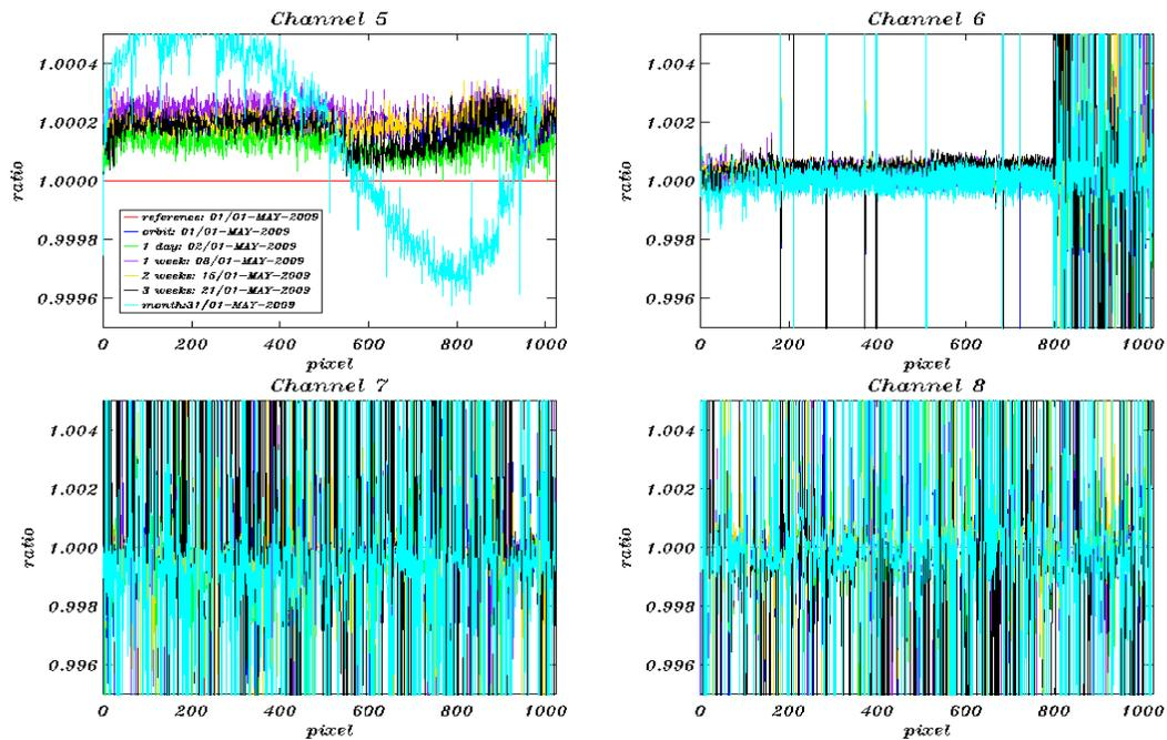
Fig. 5-9: Dark current ratios (constant part) channel 5-8 during May 2009. Reference Spectrum used: Orbit 37478, 01-May-2009.
