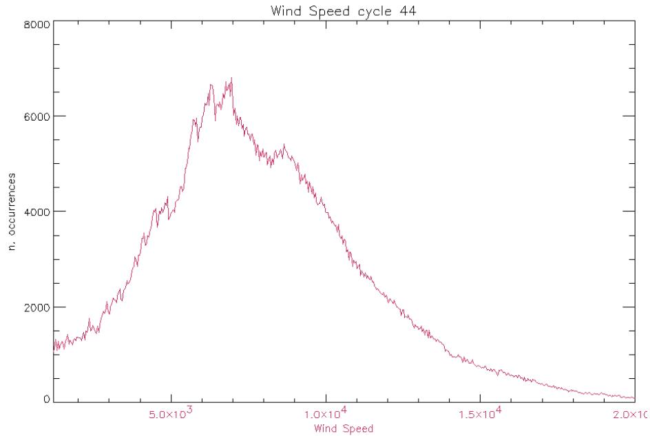
**Figure 33: Histogram of Ku Wind Speed for cycle 44 (mm/s)**
