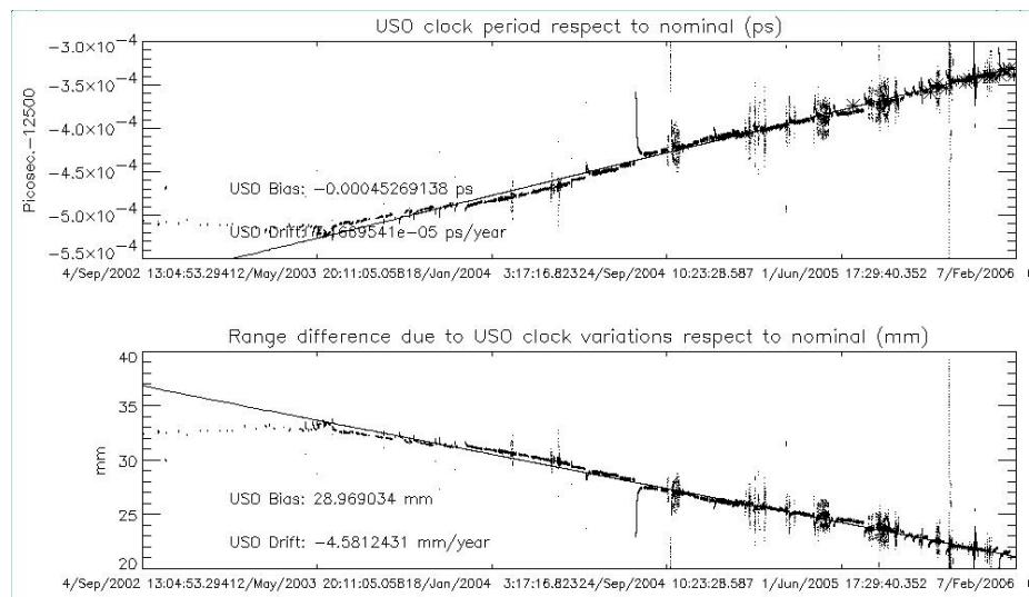
**Figure 10: USO clock period until end of cycle 44**
