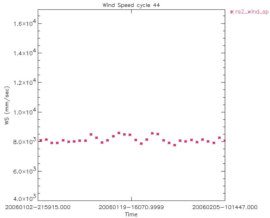
**Figure 34: Ku Band Wind Speed daily average for cycle 44 (mm/s)**
