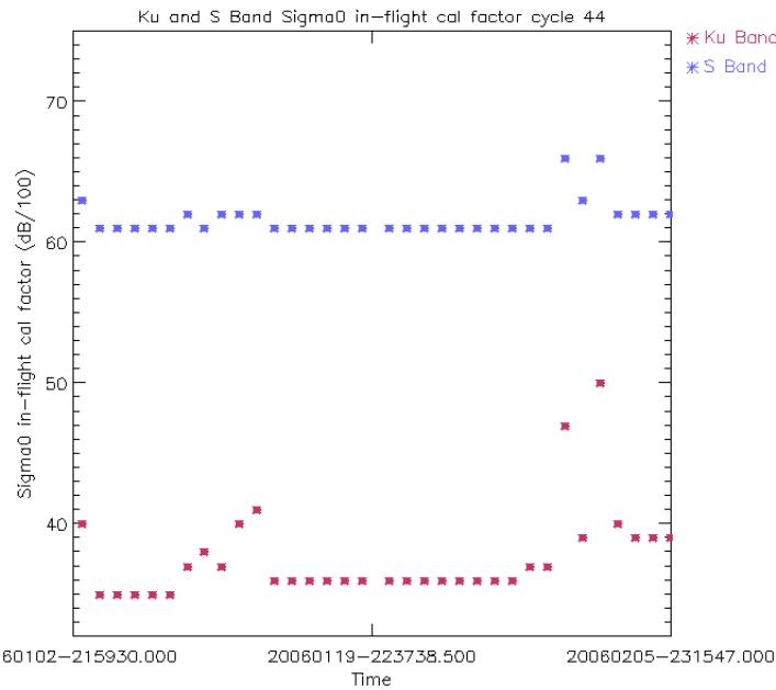
**Figure 15: Ku and S Band in-flight Sigma0 calibration factor for cycle 44**
