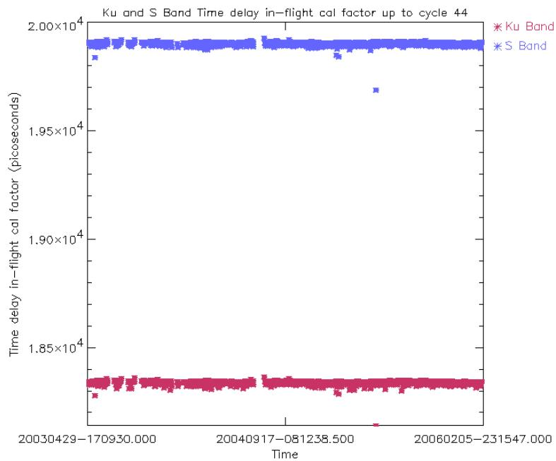
**Figure 16: Ku and S Band in-flight time delay calibration factor up to cycle 44**
