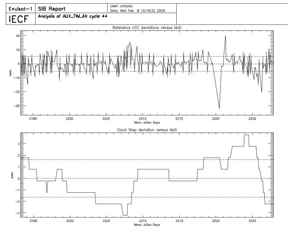
**Figure 11: UTC deviations and ICU clock period for cycle 44**
