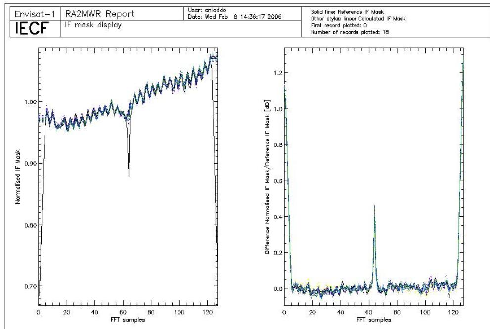
**Figure 5:** Valid IF masks retrieved daily during cycle44 plotted together with the on-ground reference.
