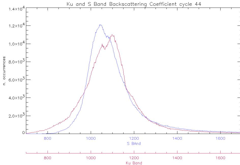
**Figure 31: Histogram of Ku and S Band Backscattering Coefficient for cycle 44 (dB/100)**
