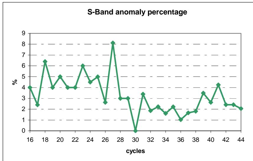
Figure 22: Percentage of data affected by the “S-Band Anomaly” for cycles 16-44
