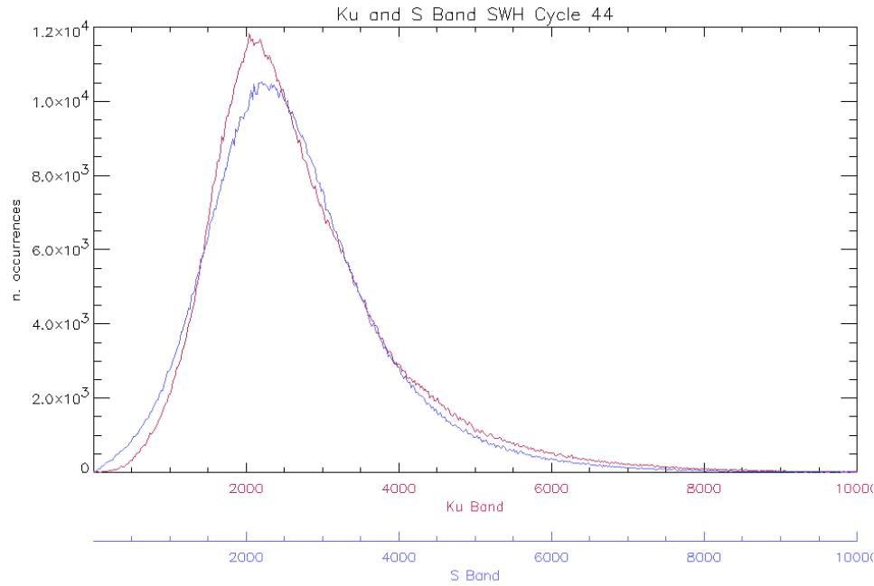
**Figure 28: Histogram of Ku and S Band SWH for cycle 44 (mm)**
