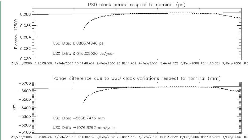
**Figure 9A: USO clock period last part of cycle 44**
