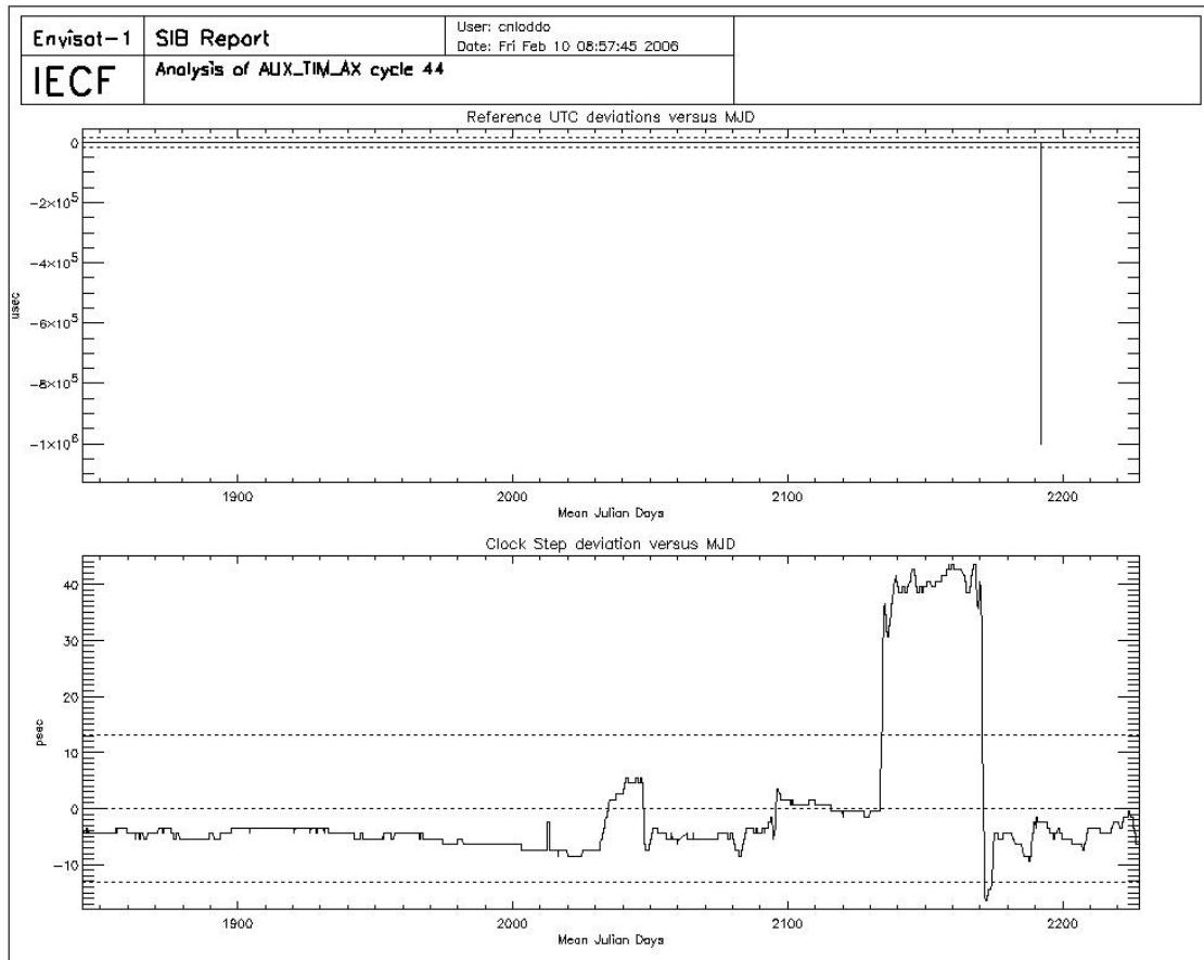
**Figure 13: UTC deviations and ICU clock period from cycle 33 up to cycle 44**
