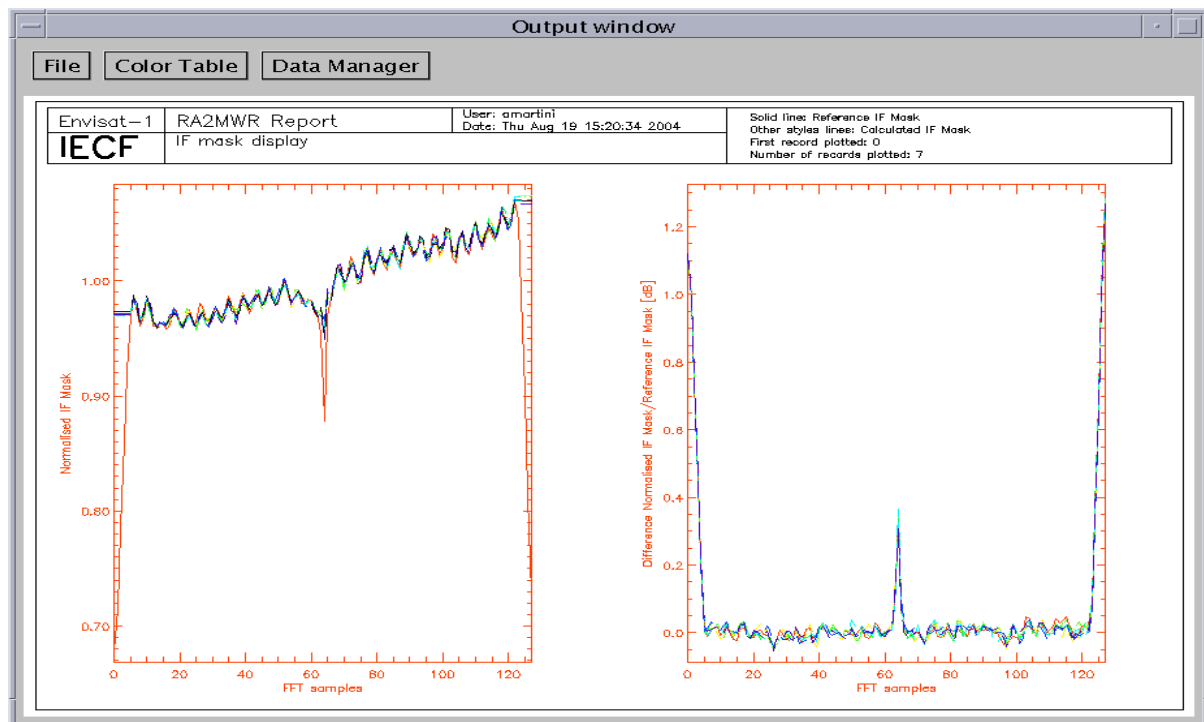
Figure 2: Valid IF masks retrieved daily during cycle 28 plotted together with the on-ground reference.
