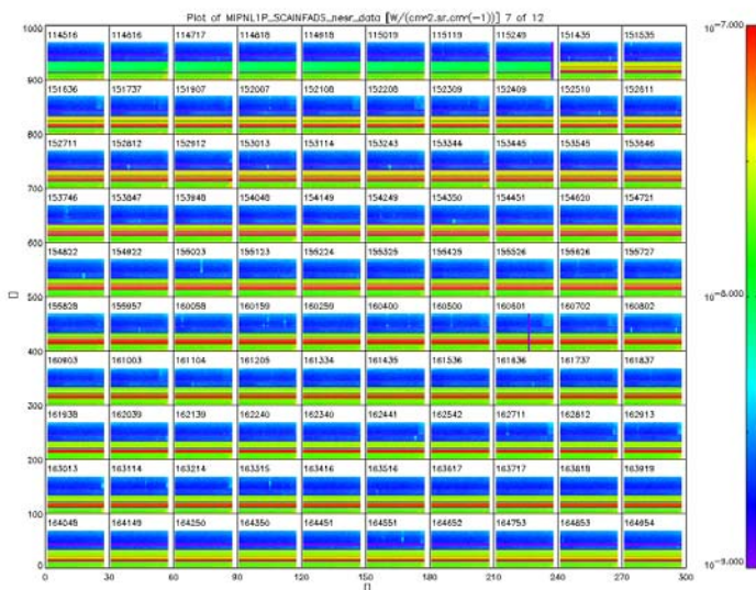
Figure 34 NESR value during 18 th Apr 2007. The red stripes show the anomaly consisting in excessive NESR values in the band AB and B.
