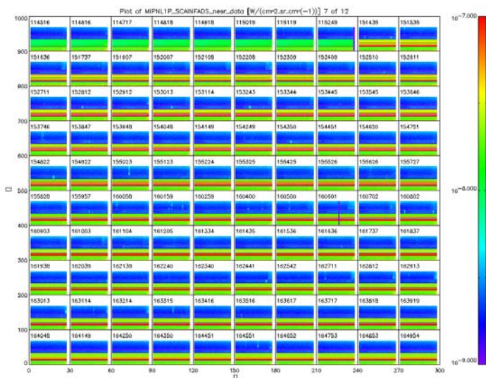
Figure 32 NESR value during 18 th Apr 2007. The red stripes show the anomaly consisting in excessive NESR values in the band AB and B.
