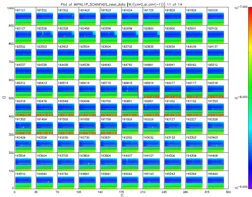
Figure 37 NESR value during 23 Jun 2008. The red stripes show the anomalous high NESR values in band A for orbit 33019.
