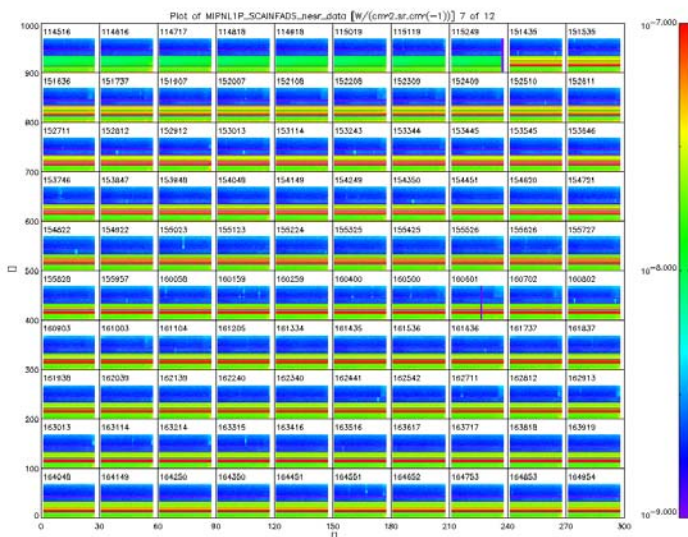
Figure 33 NESR value during 18 th Apr 2007. The red stripes show the anomaly consisting in excessive NESR values in the band AB and B.
