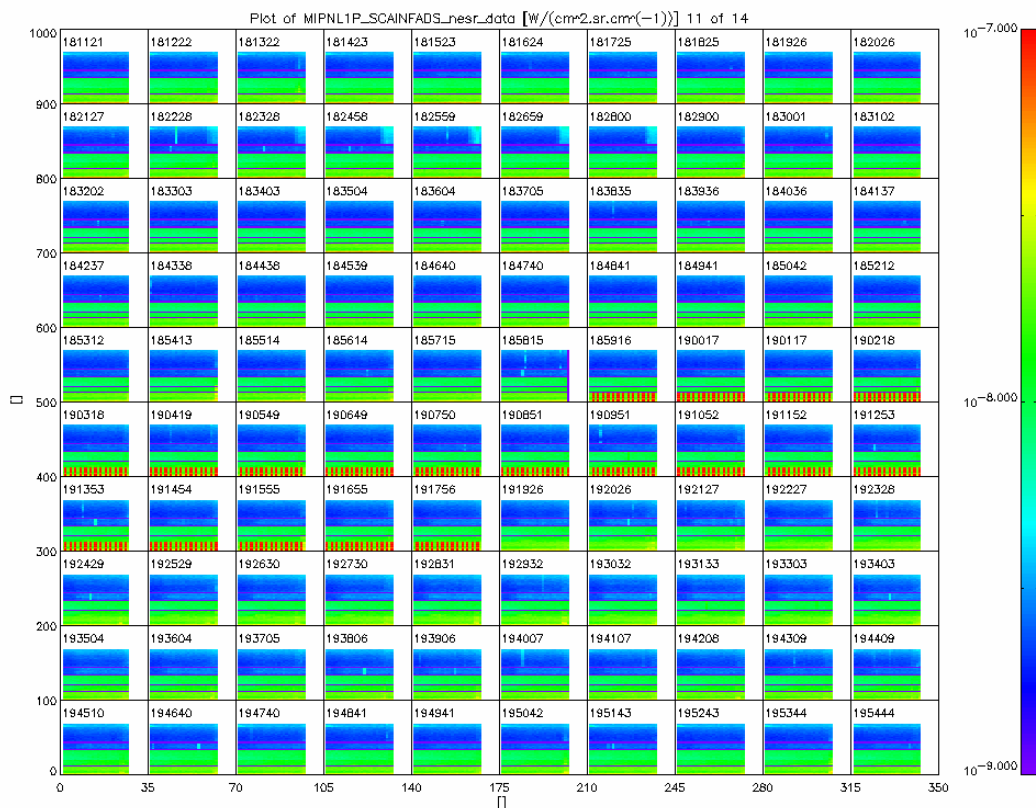
Figure 39 NESR value during 23 Jun 2008. The red stripes show the anomalous high NESR values in band A for orbit 33019.
