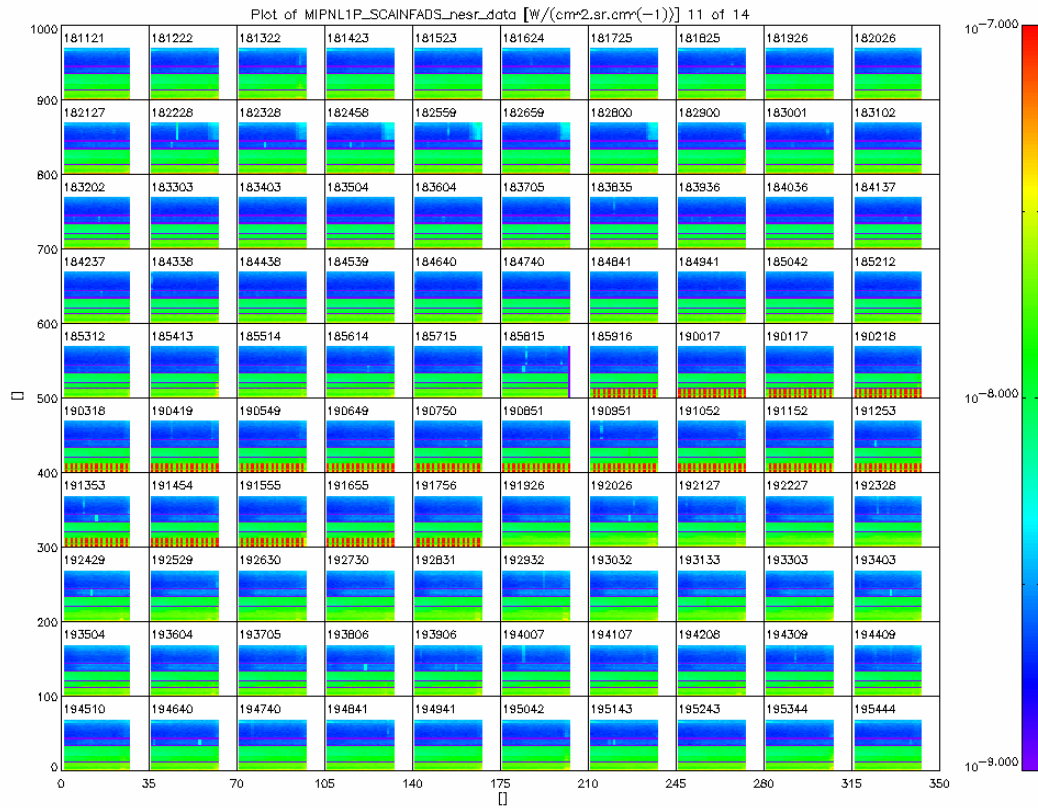
Figure 38 NESR value during 23 Jun 2008. The red stripes show the anomalous high NESR values in band A for orbit 33019.
