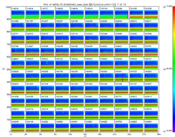
Figure 37 NCSR value during 18 th Apr 2007. The red stripes show the anomaly consisting in excessive NCSR values in the band AB and B.
