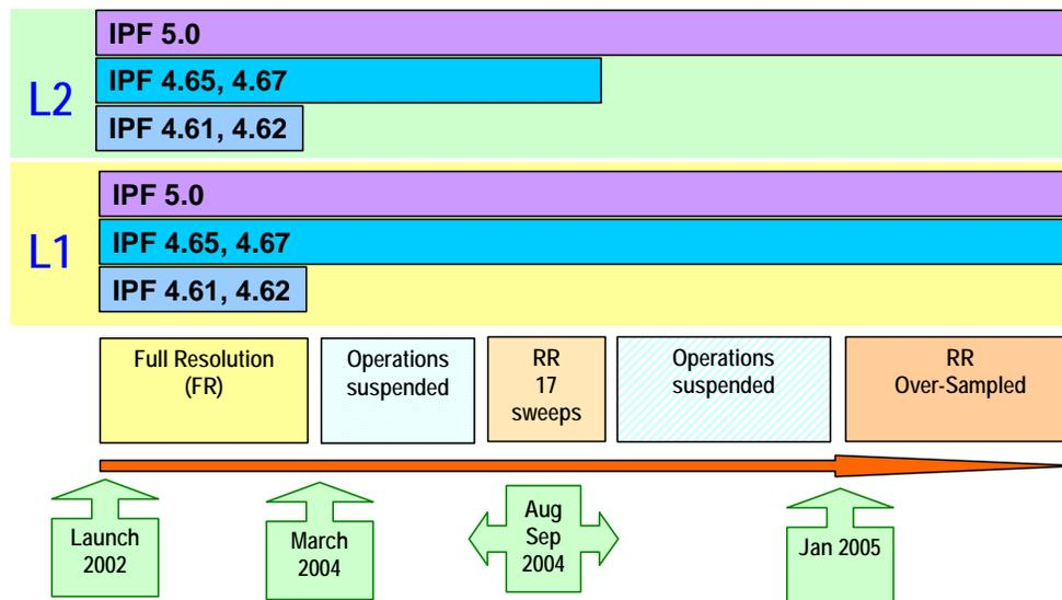
**Figure 11** IPF validity for processing level 1 and level 2 products. IPF 4.62 – 4.61 were used for re-processing of FR mission, while the IPF 4.67 is now operational at D-PAC for OFL processing of RR mission. IPF 5.0 is the future IPF that will be used for OFL processing and for reprocessing of the whole mission. IPF 5.0 will be the only one able to process RR over-sampled measurements up to L2.
