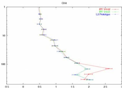
**Figure 36** Temperature N<sub>2</sub>O and CH<sub>4</sub> profiles as a function of pressure retrieved with IPF 4.62 and 4.61 compared to the prototype for seq. 16 of orbit 2975. The 4.61 profile is the reference, validated by a IMK balloon flight.
