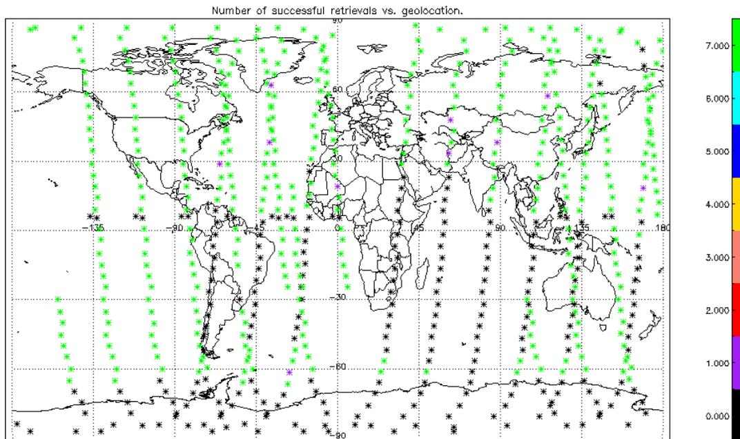
**Figure 38** MIPAS number of successful retrieval for 25 July 2002. Note that 7 is the nominal value corresponding to the target species of the ESA MIPAS products. Zero value means that the retrieval fails already at the p-T stage.
