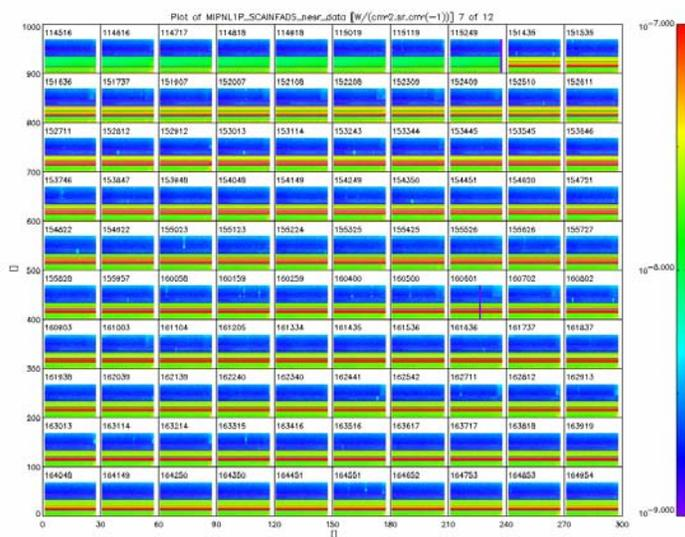
**Figure 33** NESR value during 18<sup>th</sup> Apr 2007. The red stripes show the anomaly consisting in excessive NESR values in the band AB and B.
