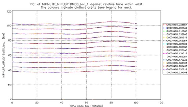
**Figure 35** Altitude of the measured sweeps as a function of ANX for the anomalous scan pattern.
