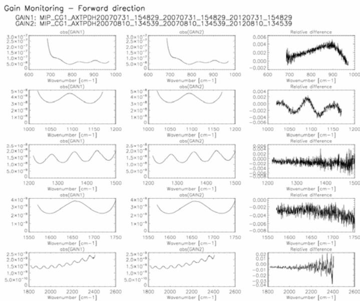
**Figure 13** Relative variations of radiometric gain for consecutive disseminated gains in band A for the forward direction. The first two plots in each row are the complex modulus of the gain for each of the 5 MIPAS bands, the third plot is the ratio:  $(abs(GAIN2) - abs(GAIN1)) / abs(GAIN1)$ . This plot refers to a gain measured on 10 Aug 2007.
