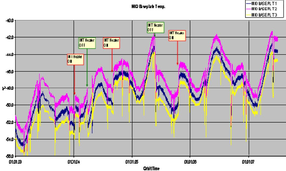
Figure 3 MIO base plate temperatures as a function of time since November 2002 (courtesy of Astrium).
