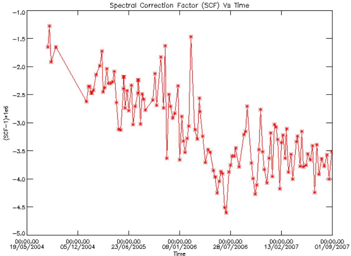
**Figure 12** MIPAS Spectral Calibration Factor (SCF) since August 2004.
