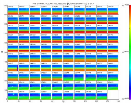
Figure 28 NESR level for different scan during 23 June 2005, each square is a scan made of 27 sweeps in nominal mode, the red lines show the anomaly of excessive high NESR, the anomaly stops when the correct ADF start to be used by the processor.
