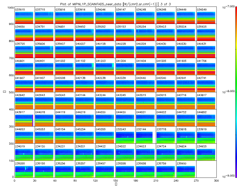
Figure 24 NESR level for different scan during 23 June 2005, each square is a scan made of 27 sweeps in nominal mode, the red lines show the anomaly of excessive high NESR, the anomaly stops when the correct ADF start to be used by the processor.
