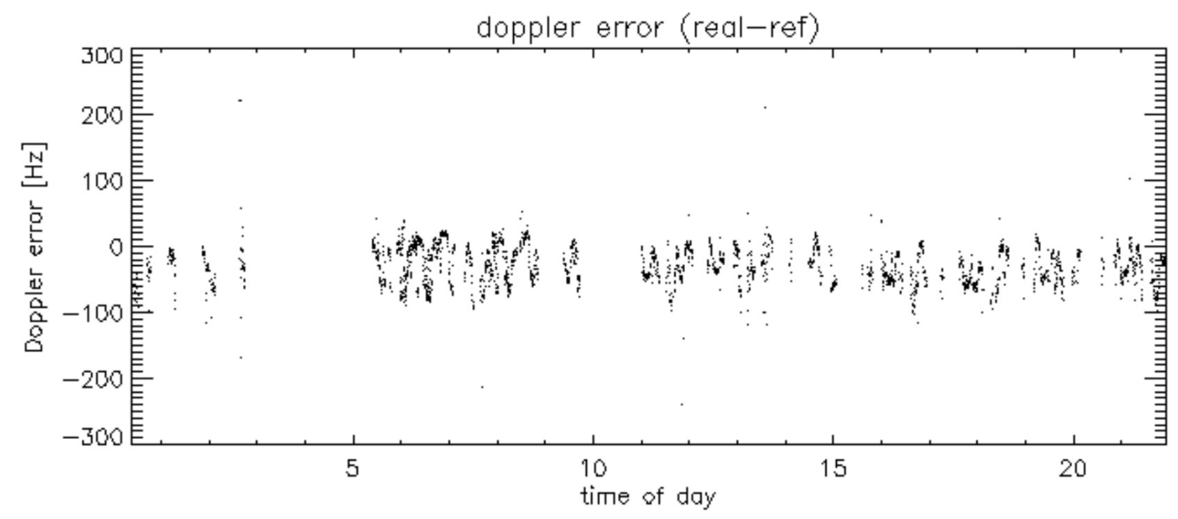
Doppler difference, estimated-predicted 'WVS' 'IS2' 'H/H' -error mean of -31.400723 Hz
