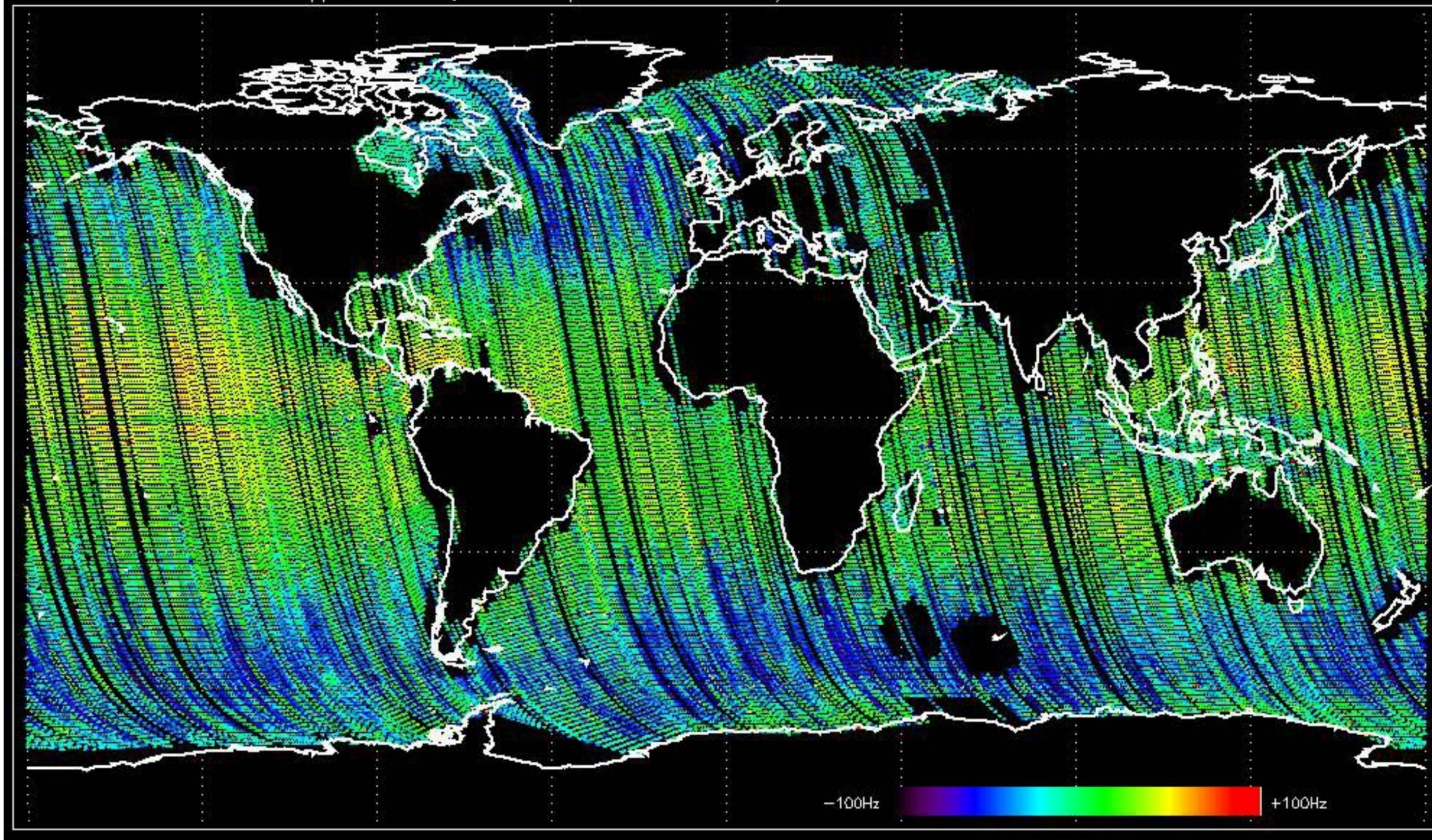
Doppler difference, estimated-predicted 'WVS' 'IS2' 'V/V' -error mean of -29.204476 Hz
