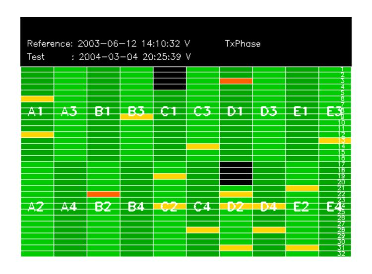
ASAR Antenna reset on 10-MAR-2004 14:36: to 14:41:24 due to OOL identifed on tile E4 on 02:55:05 to 03:00:12.
