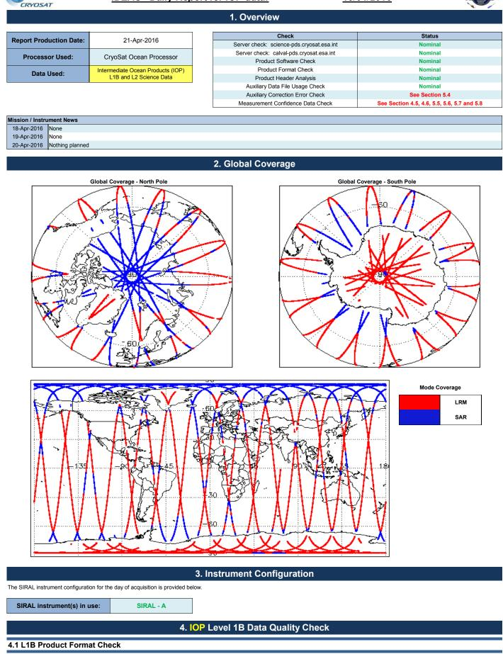
Each product, retrieved and unpacked from the science server, is checked to ensure it consists of both an XML header file (.HDR) and a binary product file (.DBL).
