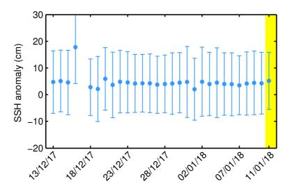
**Figure 12**. Mean science-valid SSH anomaly (blue dot) and the corresponding standard deviation (error bar) for each day in last 30-day window. The yellow shading highlights the day analyzed in this report.
