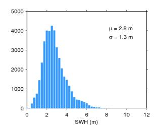
**Figure 20**. Histogram of science-valid SWH over oceans and lakes for 11/01/2018. The mean ( $\mu$ ) and standard deviation ( $\sigma$ ) are also shown. Note that values larger than 12 m are excluded from the histogram for the sake of readability but not from the computation of  $\mu$  and  $\sigma$ .
