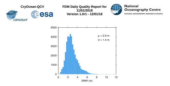
**Figure 17**. Histogram of flag-valid SWH over oceans and lakes for 11/01/2018. The mean ( $\mu$ ) and standard deviation ( $\sigma$ ) are also shown. Note that values larger than 12 m are excluded from the histogram for the sake of readability but not from the computation of  $\mu$  and  $\sigma$ .
