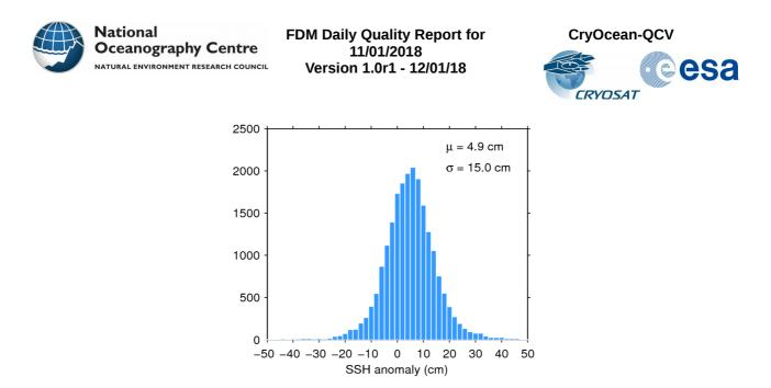
**Figure 7**. Histogram of flag-valid SSH anomaly over oceans and lakes for 11/01/2018. The mean ( $\mu$ ) and standard deviation ( $\sigma$ ) are also shown. Note that values outside [-50 50] cm are excluded from the histogram for the sake of readability but not from the computation of  $\mu$  and  $\sigma$ .
