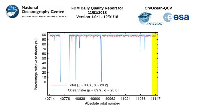
**Figure 4**. Percentage of 1-Hz records over land and ocean/lake (red) and only over ocean/lake (blue) relative to the theoretically expected number from the orbits ground tracks accounting for LRM mode mask for each orbit in last 30-day window. The yellow shading highlights the day analyzed in this report. The mean ( $\mu$ ) and standard deviation ( $\sigma$ ) are also shown.
