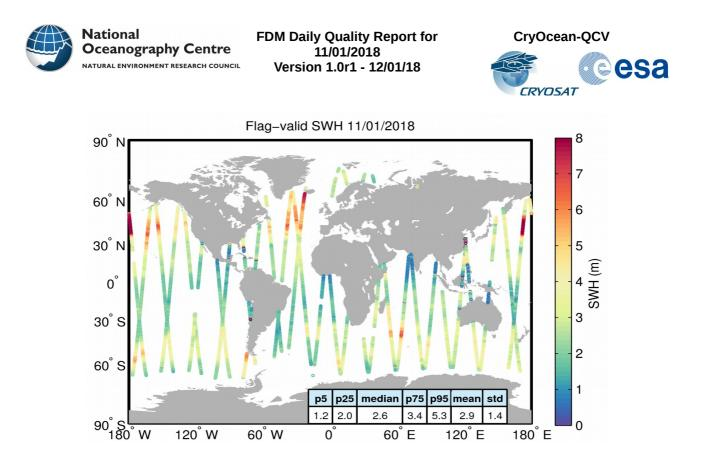
**Figure 15**. Geographical distribution of flag-valid SWH data over oceans and lakes for 11/01/2018. The statistical values shown in the table refer to the SWH in m and are calculated over all measurements shown in the figure.
