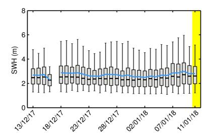
**Figure 21**. Box-and-whiskers plot for the science-valid SWH showing for each day in last 30-day window the first and third quartiles (bottom and top of the box), the median (thick black), the 5% and 95% percentiles (lower and upper whiskers), and the mean (blue). The yellow shading highlights the day analyzed in this report.
