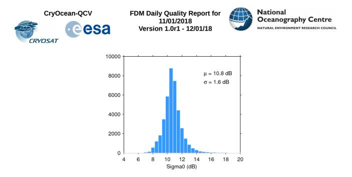
**Figure 28**. Histogram of science-valid sigma0 over oceans and lakes for 11/01/2018. The mean ( $\mu$ ) and standard deviation ( $\sigma$ ) are also shown. Note that values outside [4 20] dB are excluded from the histogram for the sake of readability but not from the computation of  $\mu$  and  $\sigma$ .
