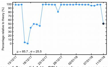
**Figure 6**. Percentage of flag-valid 1-Hz SSH records over ocean and lakes relative to theory for each day in last 30-day window. The mean ( $\mu$ ) and standard deviation ( $\sigma$ ) are also shown.
