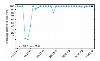
**Figure 38**. Percentage of flag-valid 1-Hz mispointing records over ocean and lakes relative to theory for each day in last 30-day window. The mean ( $\mu$ ) and standard deviation ( $\sigma$ ) are also shown.
