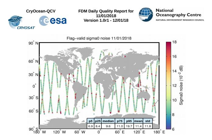
**Figure 26**. Geographical distribution of flag-valid 20-Hz sigma0 measurement noise over oceans and lakes for 11/01/2018. The statistical values shown in the table refer to the sigma0 noise and are calculated over all measurements shown in the figure.
