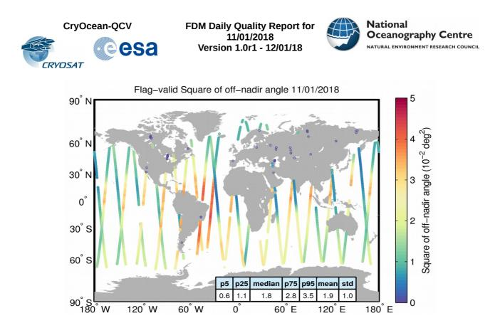
**Figure 37**. Geographical distribution of flag-valid mispointing data over oceans and lakes for 11/01/2018. The statistical values shown in the table refer to the mispointing in  $10^{-2}$  deg<sup>2</sup> and are calculated over all measurements shown in the figure.
