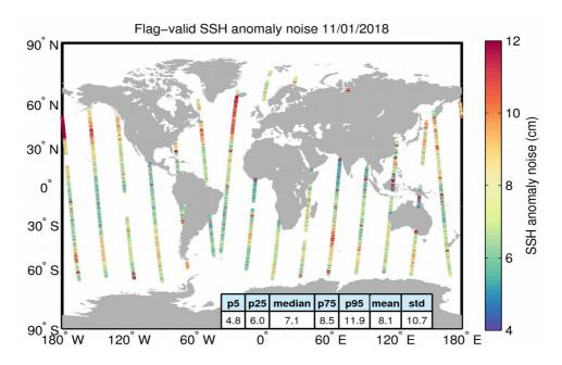
**Figure 8**. Geographical distribution of flag-valid 20-Hz SSH anomaly measurement noise over oceans and lakes for 11/01/2018. The statistical values shown in the table refer to the SSH anomaly noise and are calculated over all measurements shown in the figure.
