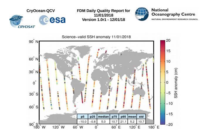
**Figure 10**. Geographical distribution of science-valid SSH anomaly data over oceans and lakes for . The statistical values shown in the table refer to the SSH anomaly in cm and are calculated over all measurements shown in the figure. Gray circles denote records that have been rejected based on the editing criteria described in Table 2.
