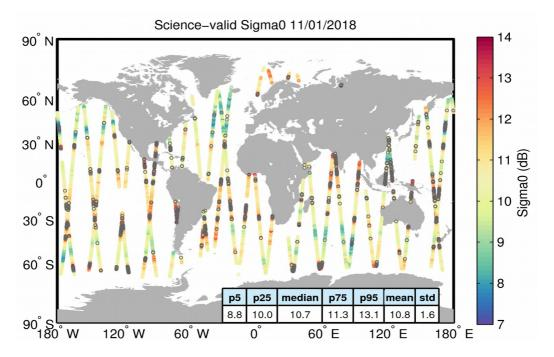
**Figure 27**. Geographical distribution of science-valid sigma0 data over oceans and lakes for 11/01/2018. The statistical values shown in the table refer to the sigma0 in dB and are calculated over all measurements shown in the figure. Gray circles denote records that have been rejected based on the editing criteria described in Table 4.
