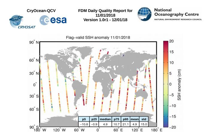
**Figure 5**. Geographical distribution of flag-valid 1-Hz SSH anomaly data over oceans and lakes for 11/01/2018. The statistical values shown in the table refer to the SSH anomaly in cm and are calculated over all measurements shown in the figure.
