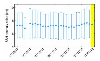
**Figure 13**. Average science-valid SSH anomaly noise (blue dot) and the corresponding standard deviation (error bar) for each day in last 30-day window. The yellow shading highlights the day analyzed in this report.
