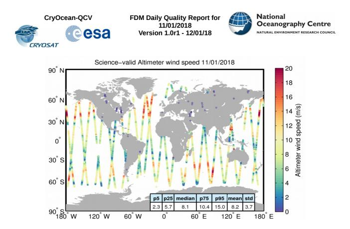
**Figure 34**. Geographical distribution of science-valid wind data over oceans and lakes for 11/01/2018. The statistical values shown in the table refer to the wind in m/s and are calculated over all measurements shown in the figure. Gray circles denote records that have been rejected based on the editing criteria described in Table 5.
