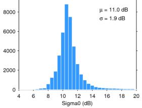
**Figure 25**. Histogram of flag-valid sigma0 over oceans and lakes for 11/01/2018. The mean ( $\mu$ ) and standard deviation ( $\sigma$ ) are also shown. Note that values outside [4 20] dB are excluded from the histogram for the sake of readability but not from the computation of  $\mu$  and  $\sigma$ .
