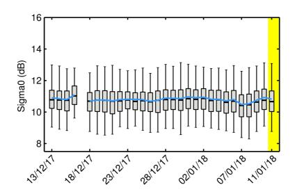
**Figure 29**. Box-and-whiskers plot for science-valid sigma0 showing for each day in last 30-day window the first and third quartiles (bottom and top of the box), the median (thick black), the 5% and 95% percentiles (lower and upper whiskers), and the mean (blue). The yellow shading highlights the day analyzed in this report.
