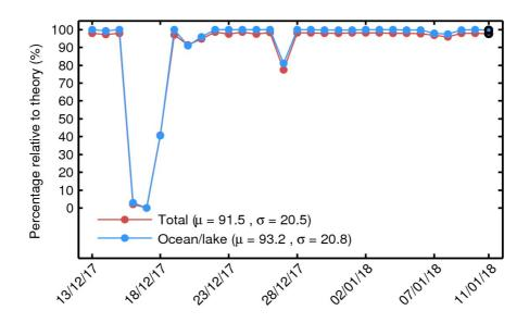
**Figure 3**. Percentage of 1-Hz records over land and ocean/lake (red) and only over ocean/lake (blue) relative to the theoretically expected number from the orbits ground tracks accounting for LRM mode mask for each day in last 30-day window. The black circle at the end of the time series highlights the day analyzed in this report.
