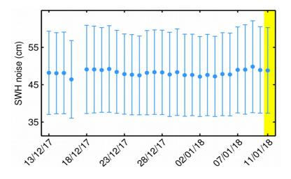
**Figure 22**. Average science-valid SWH noise (blue dot) and the corresponding standard deviation (error bar) for each day in last 30-day window. The yellow shading highlights the day analyzed in this report.
