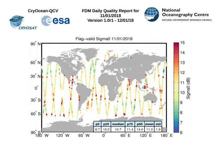
**Figure 23**. Geographical distribution of flag-valid sigma0 data over oceans and lakes for 11/01/2018. The statistical values shown in the table refer to the sigma0 in dB and are calculated over all measurements shown in the figure.
