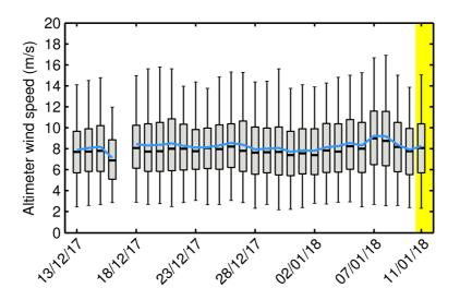
**Figure 36**. Box-and-whiskers plot for the science-valid wind showing for each day in last 30-day window the first and third quartiles (bottom and top of the box), the median (thick black), the 5% and 95% percentiles (lower and upper whiskers), and the mean (blue). The yellow shading highlights the day analyzed in this report.
