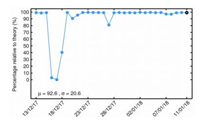
**Figure 24**. Percentage of flag-valid 1-Hz sigma0 records over ocean and lakes relative to theory for each day in last 30-day window. The mean ( $\mu$ ) and standard deviation ( $\sigma$ ) are also shown.
