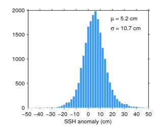
**Figure 11**. Histogram of science-valid SSH anomaly over oceans and lakes for 11/01/2018. The mean ( $\mu$ ) and standard deviation ( $\sigma$ ) are also shown. Note that values outside [-50 50] cm are excluded from the histogram for the sake of readability but not from the computation of  $\mu$  and  $\sigma$ .
