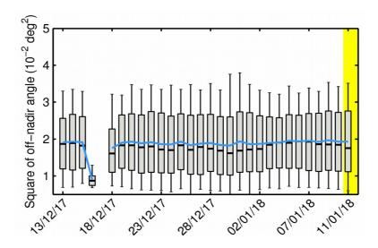
**Figure 40**. Box-and-whiskers plot for flag-valid mispointing showing for each day in last 30-day window the first and third quartiles (bottom and top of the box), the median (thick black), the 5% and 95% percentiles (lower and upper whiskers), and the mean (blue). The yellow shading highlights the day analyzed in this report.
