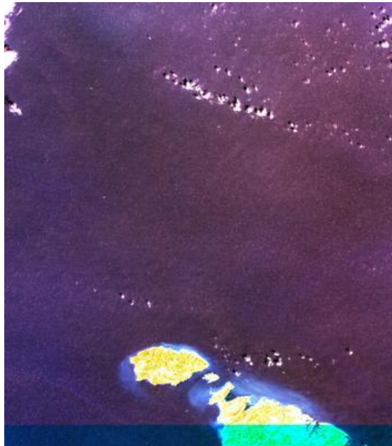
Figure 5-1 Level 1B1 AVNIR-2 image from frame 2880, orbit 11543 which shows missing data in one band towards the bottom of the image.
